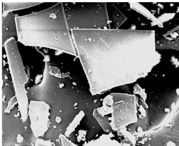
Fig. 5. SEM image of [\text{H}_3\text{N}(\text{CH}_2)_6\text{NH}_3]_2\text{AlX}_7\cdot\text{H}_2\text{O} ( \text{X} = \text{F}, \text{OH} ) crystals.
